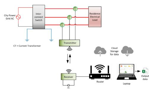
**Fig. 2.** Schematic diagram for the layout of the energy monitoring system The figure descriptively explains how the energy monitoring system was connected and how data was exchanged.
