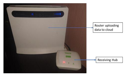
Fig. 5. Energy consumption data receiver and uploading to cloud system
