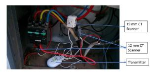
Fig. 4. CT scanners and transmitter The figure shows the experimental set-up at the student residence.
